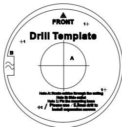
Figure 2-4 Drill Holes on the Ceiling
